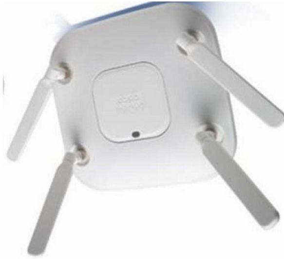
Figure 9-1 AP With Antennas Arranged (incorrectly) in Different Directions
