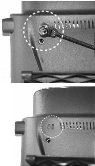
Figure 1: Connecting a Cable Lock to the Cisco Unified IP Phone
