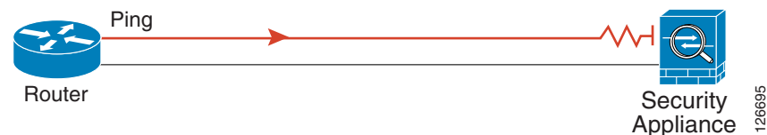
Figure 79-2 Ping Failure at Security Appliance Interface
