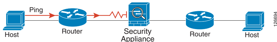
Figure 79-5 Ping Failure Because the Security Appliance is not Translating Addresses
