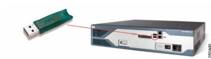
Figure 29 Aladdin Knowledge Systems USB eToken and Cisco ISR
