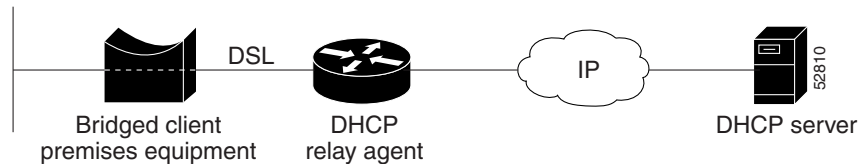
Figure 15 Network Topology Using ATM RBE and DHCP
