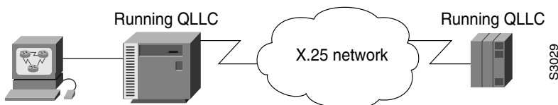
Figure 163 SNA Devices Running QLLC
