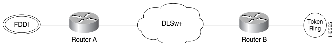
Figure 136 DLSw+ Translation Between FDDI and Token Ring
