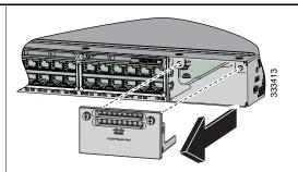
Slide the network module into the opening until the back of the module faceplate is flush with the switch faceplate. Tighten the captive screws. For a list of supported network modules, see the *Catalyst 3850 Switch Hardware Installation Guide* at:
