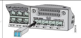
**Step 2** Connect an appropriate cable to the module port.
