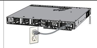
Step 5 Observe the POST results. Approximately 30 seconds after the switch powers on, it begins the power-on self-test (POST), which can take up to 5 minutes to complete.
