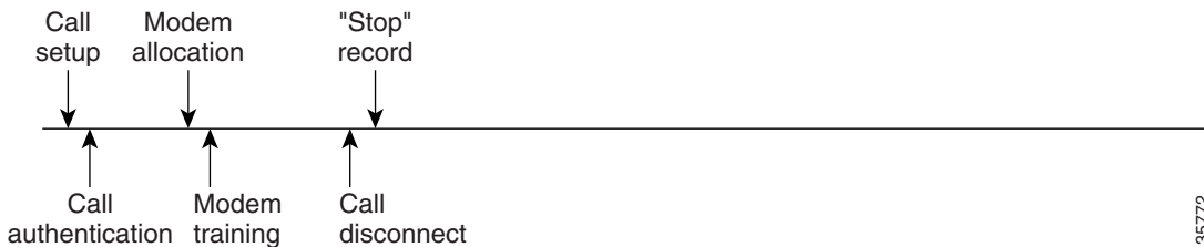
Figure 10 Modem Dial-In Call Setup Sequence With Call Disconnect Occurring Before User Authentication and With Resource Failure Stop Accounting Enabled
