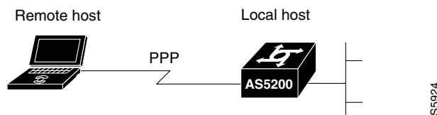
Figure 2 Network Topology for Activating Double Authentication (Example)
