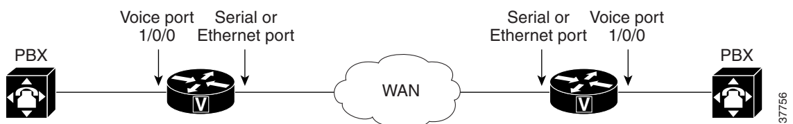
Figure 12 PBX-to-PBX over a WAN
