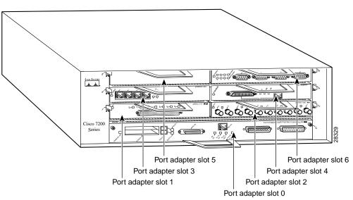
Figure 1-21 Module Slots in the Cisco 7206
