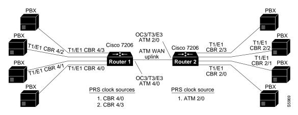
Each PRS depicted in Figure 1-6 is externally generated—that is, the timing signal originates from a source outside the router. Also shown is an OC-3 trunk line that can propagate a PRS between adjacent router/network devices.
