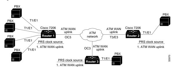
Figure 1-7 Cisco 7206 Routers Connected to ATM Network
