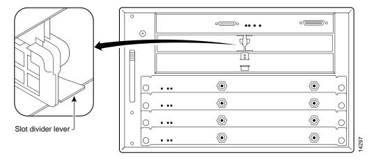
Figure 3-2 Slot Divider Lever—Cisco uBR7246 Shown
