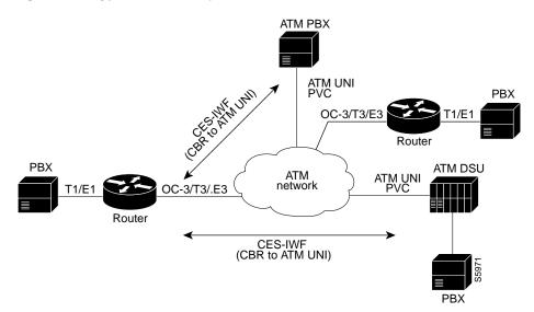
Figure 1-1 Typical CES-IWF Operations in an ATM Network
