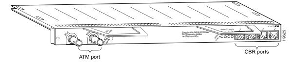
You can install a PA-A2 ATM CES port adapter in any available, horizontally aligned, port of port adapter slots in a Cisco 7200 series router or a Cisco uBR7246.
