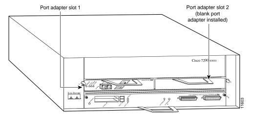
Slots in the Cisco 7204 router are numbered from left to right, beginning with slot 1 and continuing through slot 4. Slot 0 is the Fast Ethernet port on the I/O controller. (See Figure 1-20.)
