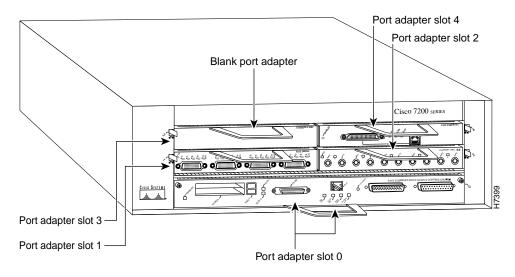
Slots in the Cisco 7206 are numbered from 1 through 6; slot 0 is reserved for the optional Fast Ethernet port on the I/O controller—if present. (See Figure 1-21.)
