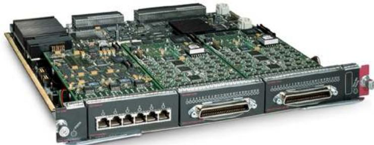
The Cisco CMM is a modular line card that supports four different types of port adapters, including 6-port T1, 6-port E1, 24-port foreign exchange station (FXS), and 128-port conferencing and transcoding port adapters. Up to four port adapters can be installed in a single Cisco CMM Line Card. Customers have the flexibility of mixing any of the four types of port adapters in a single Cisco CMM (Note: Mixed E1 and T1 port adapters on the same CMM are not allowed).
