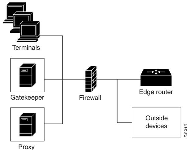
Because the gatekeeper (using RAS) and the proxy (using call setup protocols) are the only endpoints that communicate with other devices outside the firewall, it is simple to set up a tunnel through the firewall to allow traffic destined for either of these two endpoints to pass through.
