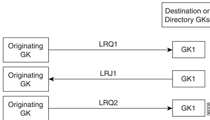
Figure 12 shows a call flow with the Sequential LRQ Enhancement feature when LRJ1 arrives after the delay timer has expired and after LRQ2 has been sent. If this occurs, the originating gatekeeper does not send LRQ3 and ignores LRQ2.
