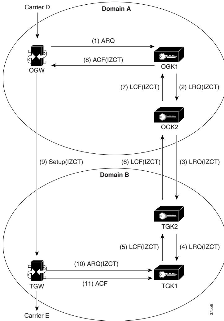
1. The originating gateway sends an ARQ message with an interface description as a nonstandard field to originating gatekeeper 1 (OGK1). The interface description is treated as a source carrier identifier.
