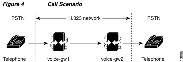
Additionally, in using the **gw-type-prefix** command, a particular gateway-type prefix can be defined as the default gateway type to be used for addresses that cannot be resolved. It also forces a technology prefix to always hop off in a particular zone.
