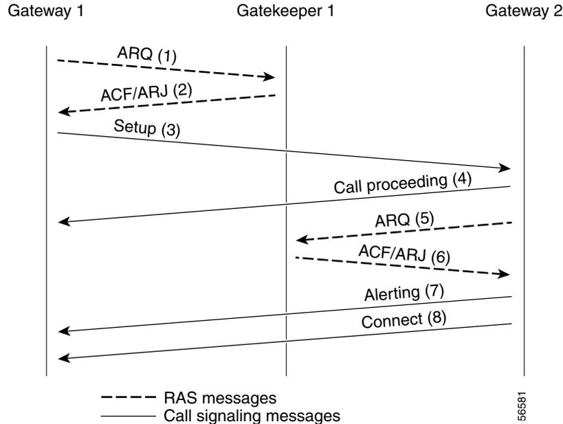
Fast connect allows endpoints to establish media channels without waiting for a separate H.245 connection to be opened. This streamlines the number of messages that are exchanged and the amount of processing that must be done before endpoint connections can be established. A high-level view of the fast-connect procedures within the H.323 protocol follows:
