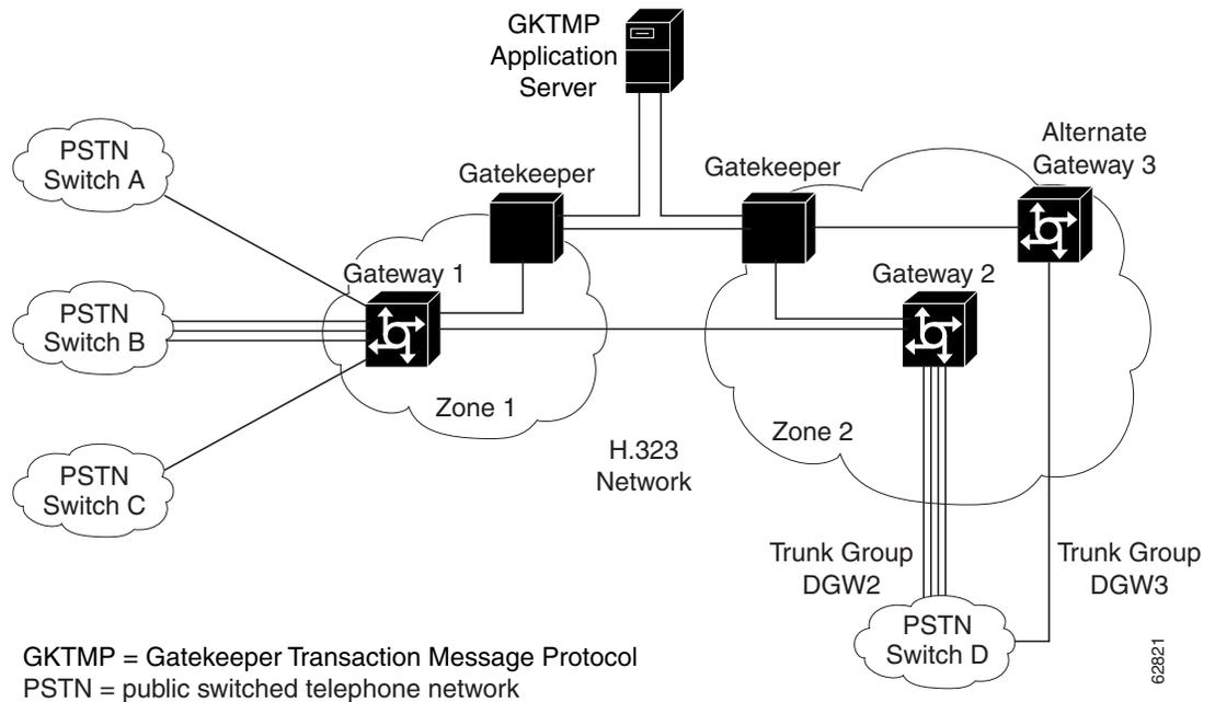
The RAS message includes a new field called circuitInfo. The information in the circuitInfo field corresponds to the information in the Q and J tags in the GKTMP message. The trunk group label (Q tag) or carrier ID (J tag) of the primary gateway is provided in the alternateEndpoint structure of the GKTMP message, along with the call signal address of the primary gateway. The trunk group label or
