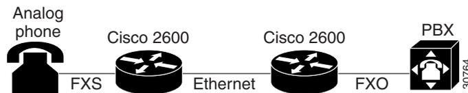
In Cisco H.323 Version 2 software, an FXS hookflash relay is generated only if the following two conditions are met:
