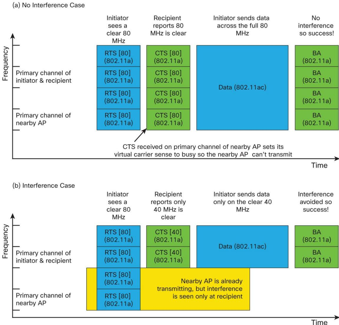
For this reason, 802.11ac defines an enhanced RTS/CTS protocol. RTS/CTS can be used to determine when channel bandwidth is clear and how much, around both the initiator and the responder, as shown in [Figure 3](#).
