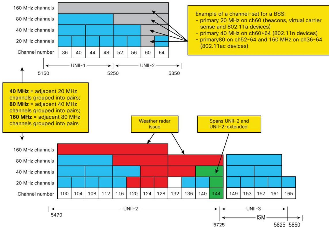
In the United States, there are 20 to 25 20-MHz channels, 8 to 12 40-MHz channels, 4 to 6 80-MHz channels, and 1 or 2 160-MHz channels. These numbers are ranges because of the evolving regulatory issues surrounding the different spectrum noted in [Figure 4](#).
